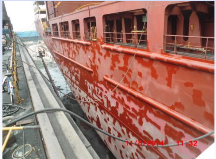
Sandblasted and first coat painted
