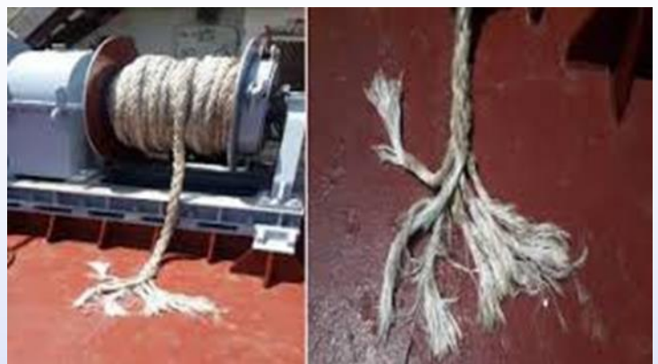
Every Masters nightmare, broken mooring lines
